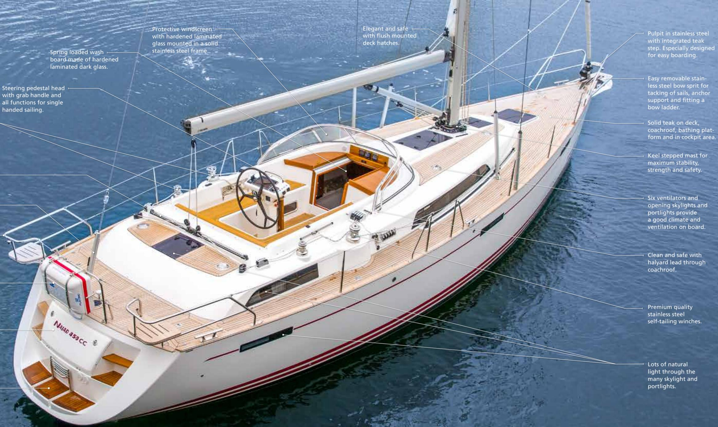
Spring loaded wash board made of hardened laminated dark glass.
